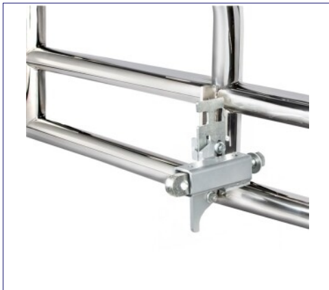
Item No. 80004 Grille Guard Mounting Bracket Set For 2004-2017 Volvo VNL MSRP: $ 293.59 OEM No. :
